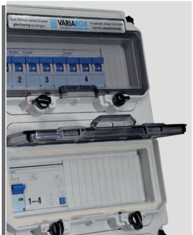
The operating window with the unique OTC mechanism (One Touch Close) engages in the open state and automatically closes and locks again when touched lightly
