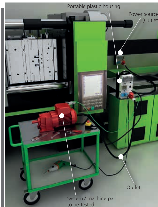
Non-stationary test system - portable plastic housing
